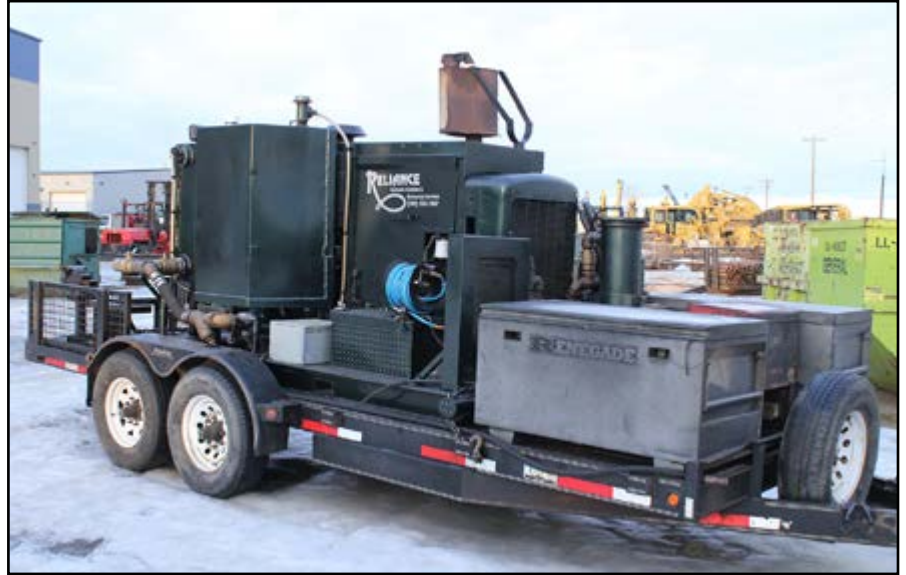
Flushing Unit consists of oilfield skid mounted on an 18-ft trailer for easy transport.
